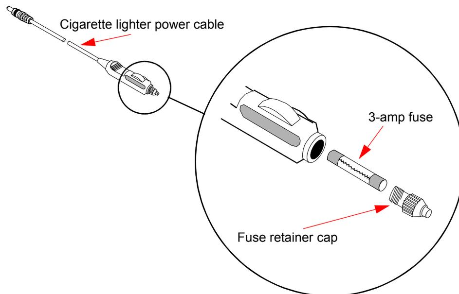
FIGURE 6-17. Cigarette Lighter Power Cable 3-Amp Fuse Replacement
