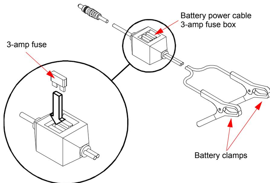
FIGURE 6-18. Battery Power Cable 3-Amp Fuse Replacement
