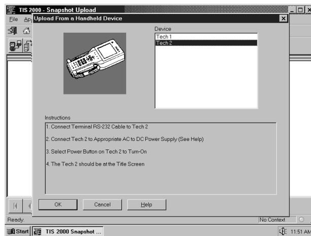
FIGURE 8-39. Upload from a Handheld Device Screen
