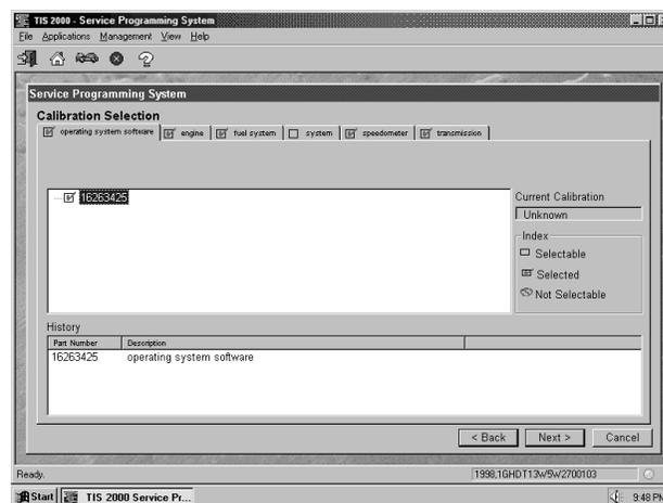
FIGURE 8-26. Operating System Software Folder on Calibration Selection Screen
