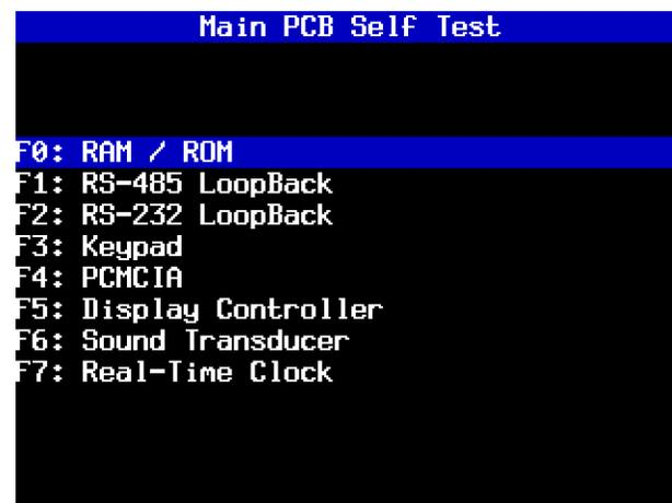
FIGURE 6-12. Selectable Main PCB Self Test Screen
