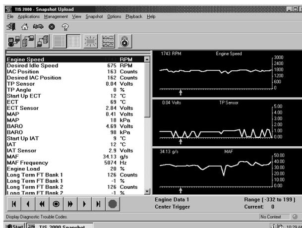
FIGURE 8-47. Three Parameters Shown in Graph Form
