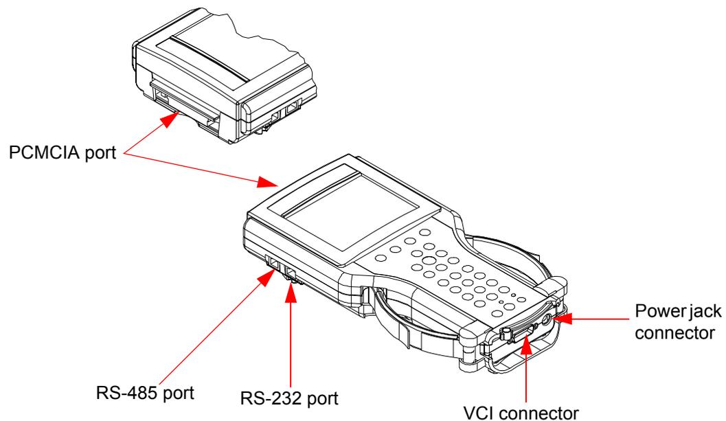
FIGURE 3-1. Identification of the Tech 2's External Ports
