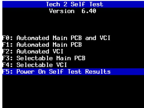
FIGURE 6-16. Power On Self Test Results Selected on Tech 2 Self Test Main Menu
