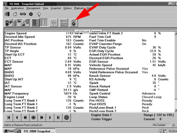
FIGURE 8-49. Lock/Unlock Parameters Icon on SSnapshot Upload Screen
