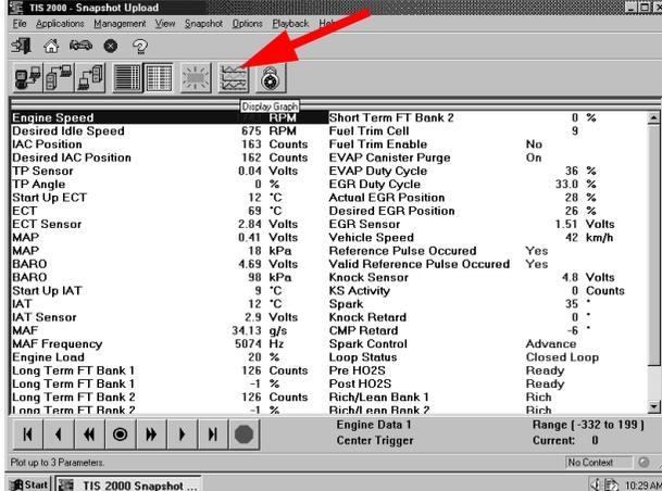
FIGURE 8-45. Display Graph Icon on Snapshot Upload Screen
