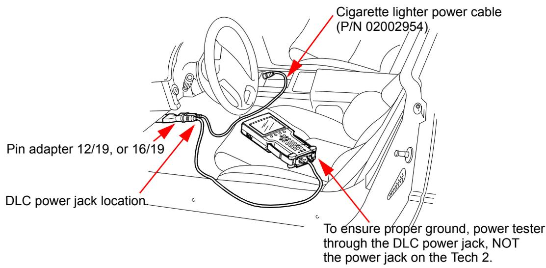
FIGURE 3-24. Attaching the Tech 2 to Non-OBD II-Equipped Vehicles
