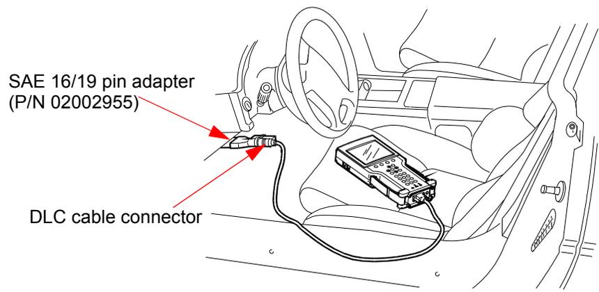
FIGURE 3-23. Attaching the Tech 2 to OBD II-Equipped Vehicles
