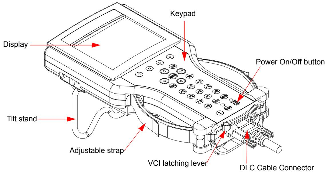
FIGURE 1-1. External Features of the Tech 2 (Front View)
