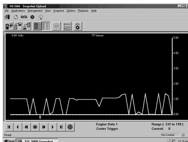
FIGURE 8-48. TP Sensor Parameter Shown in Full-Size Graph
