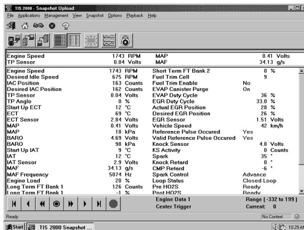
FIGURE 8-50. Snapshot Upload Screen Showing “Locked” List
