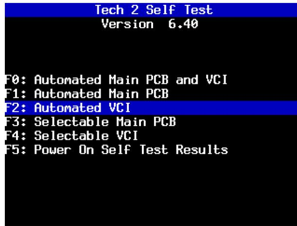
FIGURE 6-10. Automated VCI Test Selected on Tech 2 Self Test Main Menu
