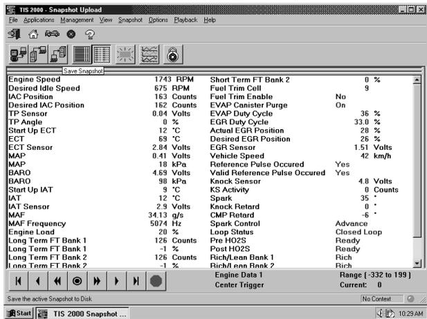
FIGURE 8-53. Save Snapshot Icon on Snapshot Upload Screen
