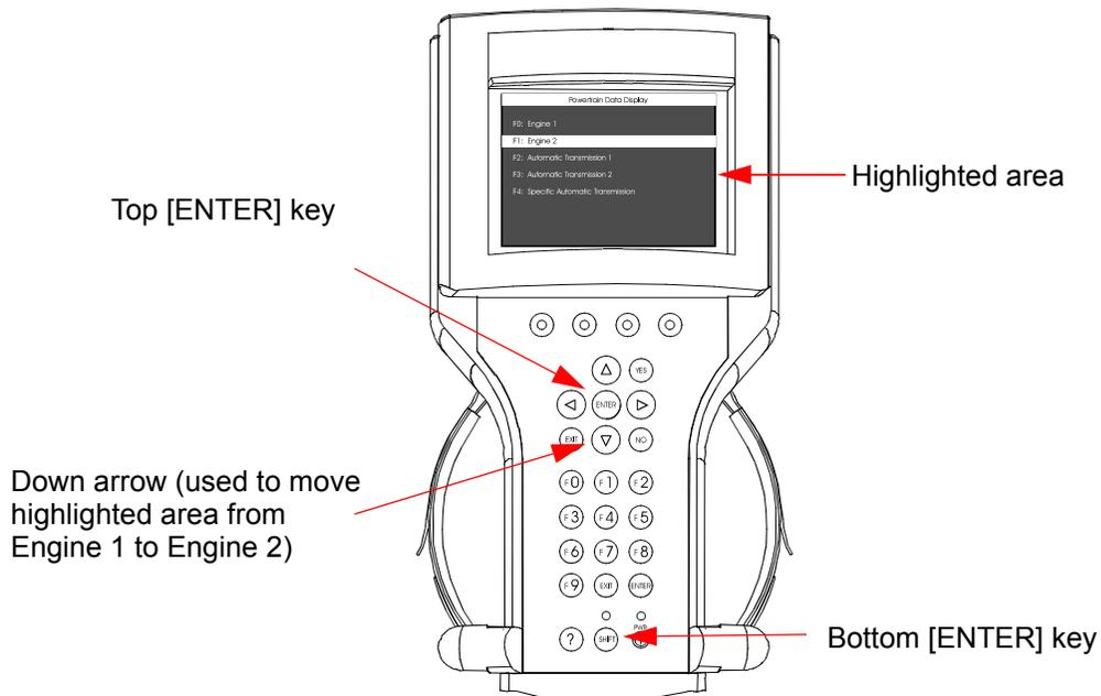
FIGURE 3-19. Positioning Highlighted Area to Make a Selection
