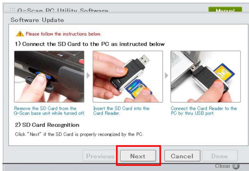
[Fig. 2] SD Card inserted to PC
