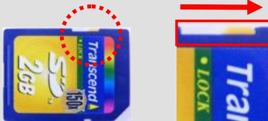
[Fig. 2] SD Card Write Protection Tab
