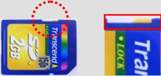
**[Fig. 3] SD Card Write Protection Tab**
