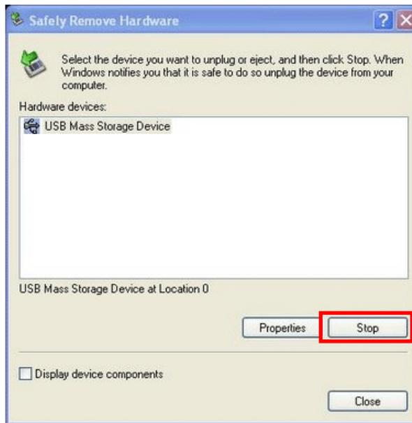
**[Fig. 8] Stop use of USB Mass Storage Device**
