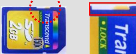
[Fig. 4] SD Card Write Protection Tab
