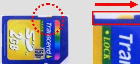
[Fig. 2] SD Card Write Protection Tab
