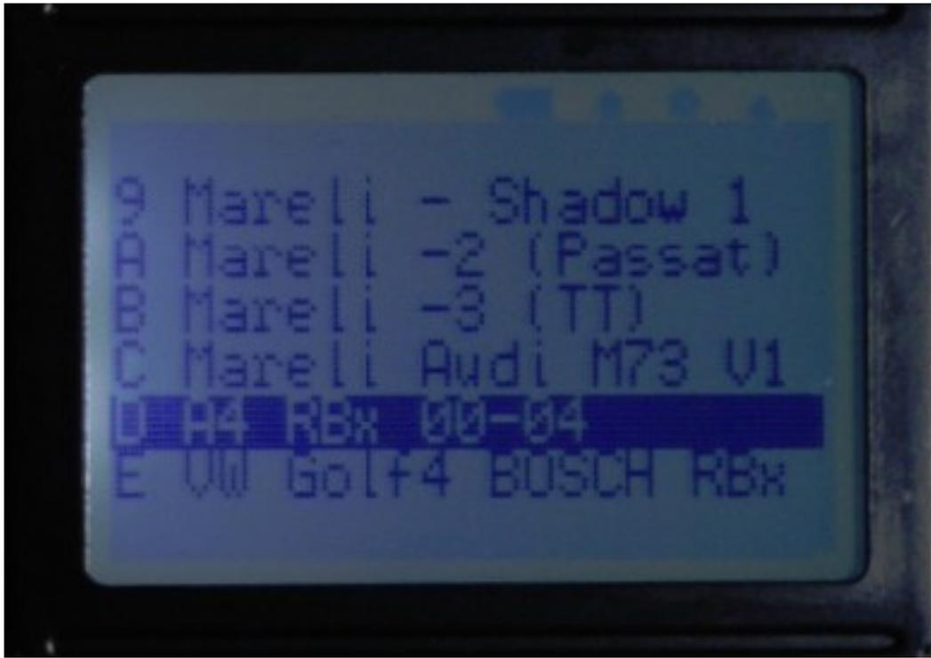
According to the type of odometer, select the corresponding option. Maily odometer is divided into K line and CAN line, but the K line and CAN have different manufacturers, different versions, different types of odometer. User can choose K-line or CAN line automatic way, for some special odometer, user select the corresponding instrument through the menu.
