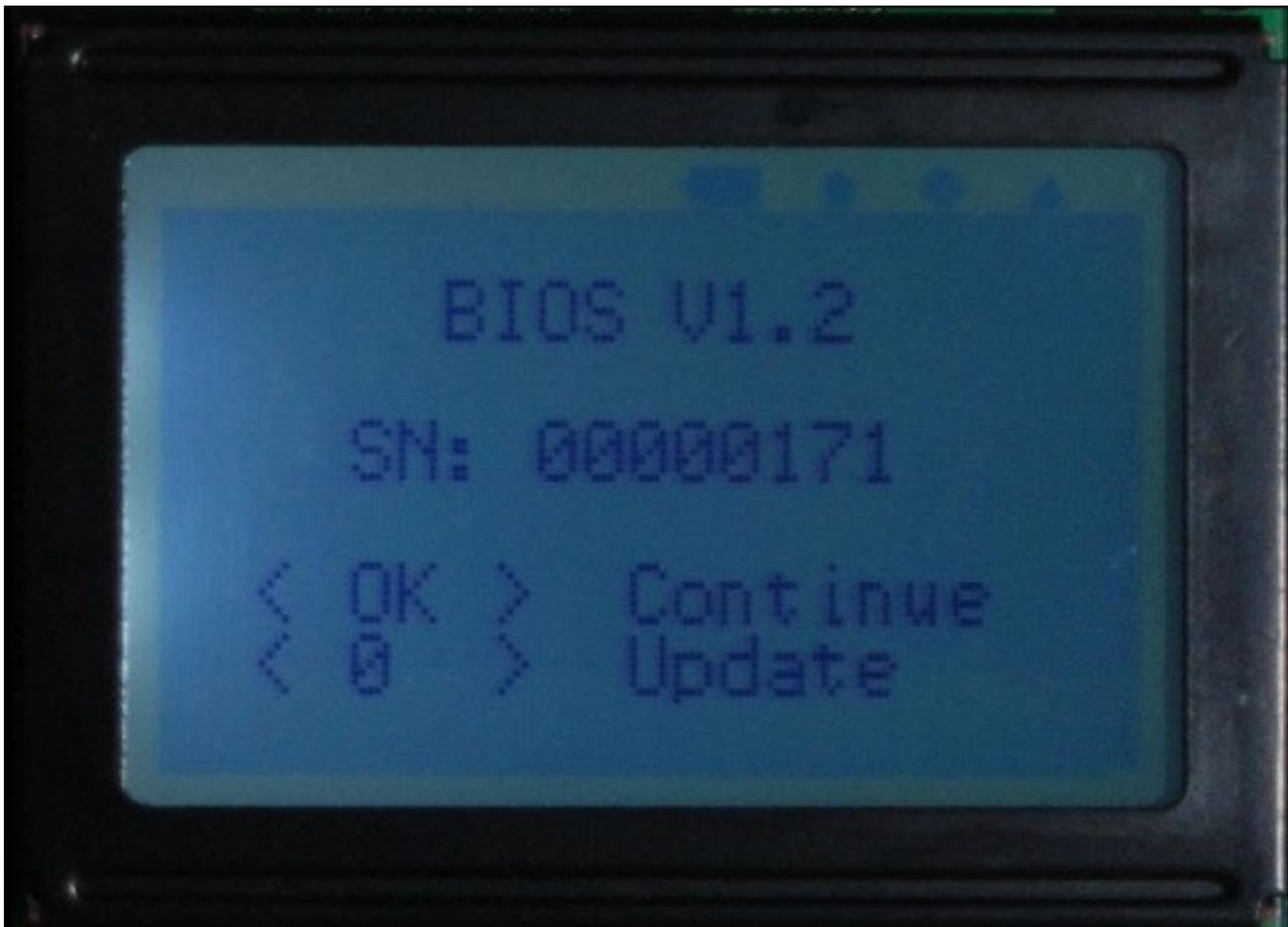
Input 0 in keyboard, when appear the following interface, it means the device has entered the state to upgrade.
