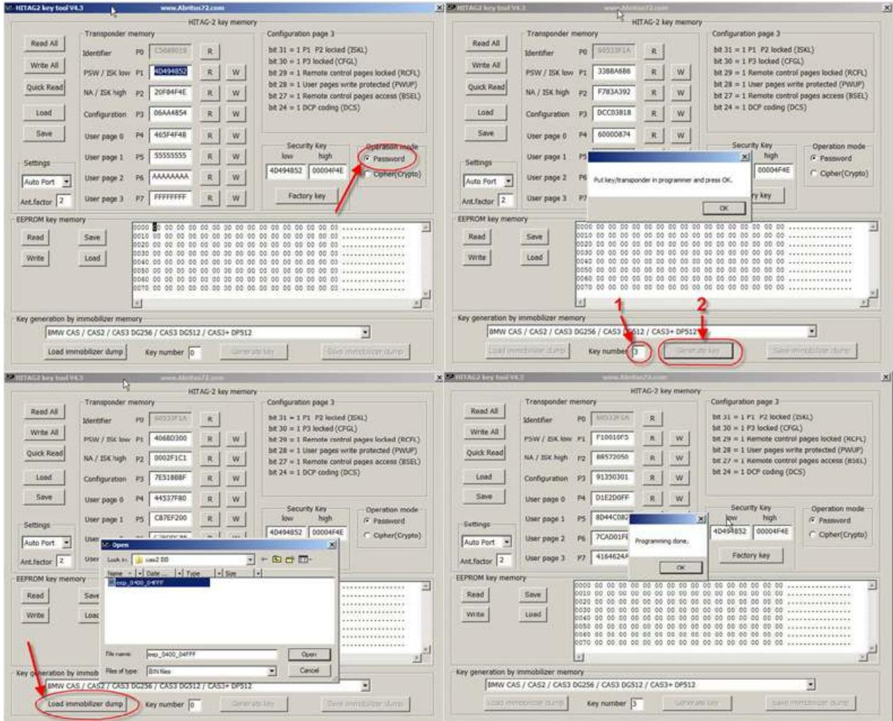
**Attached picture is EXAMPLE how to programm transponder - BMW E60 with CAS2.**
