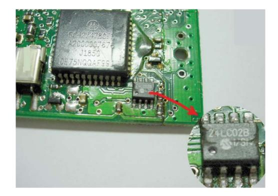
4. Clear every pin of 24LC02B and connect the clips with microchip , Black point to pin1 of 24LC02B .
