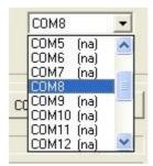
As you see in the image, next to COM's there is (na). This means that your device is not connected to that COM. If there is a COM that does not have na, then this is the COM that your device is connected to. In the image we see that your device is connected to COM8. You should select COM8 to connect it to our device.
