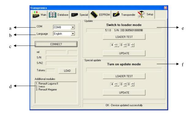
After you connect your device to your computer, you have make adjustment in COM. Our pc software can detect which COM is used.
