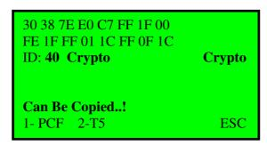
This shows that only the transponder's ID part can be copied, when you see this ,there is no probability to start the car. And the ID 40 transponder, which is in the example, is locked and can not be identified to another car with another device
