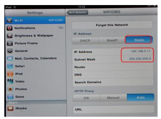
Scan for the WiFiOBD device, and join the network.
