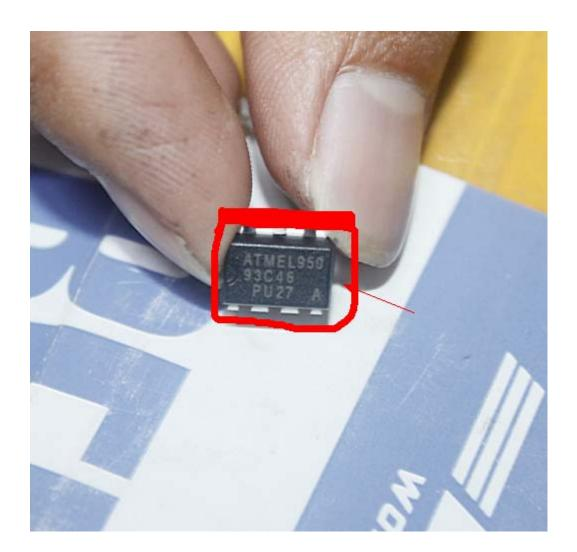
10, insert the chip in the right position and connect the OBP, (Note: notice 93C46 direction)
