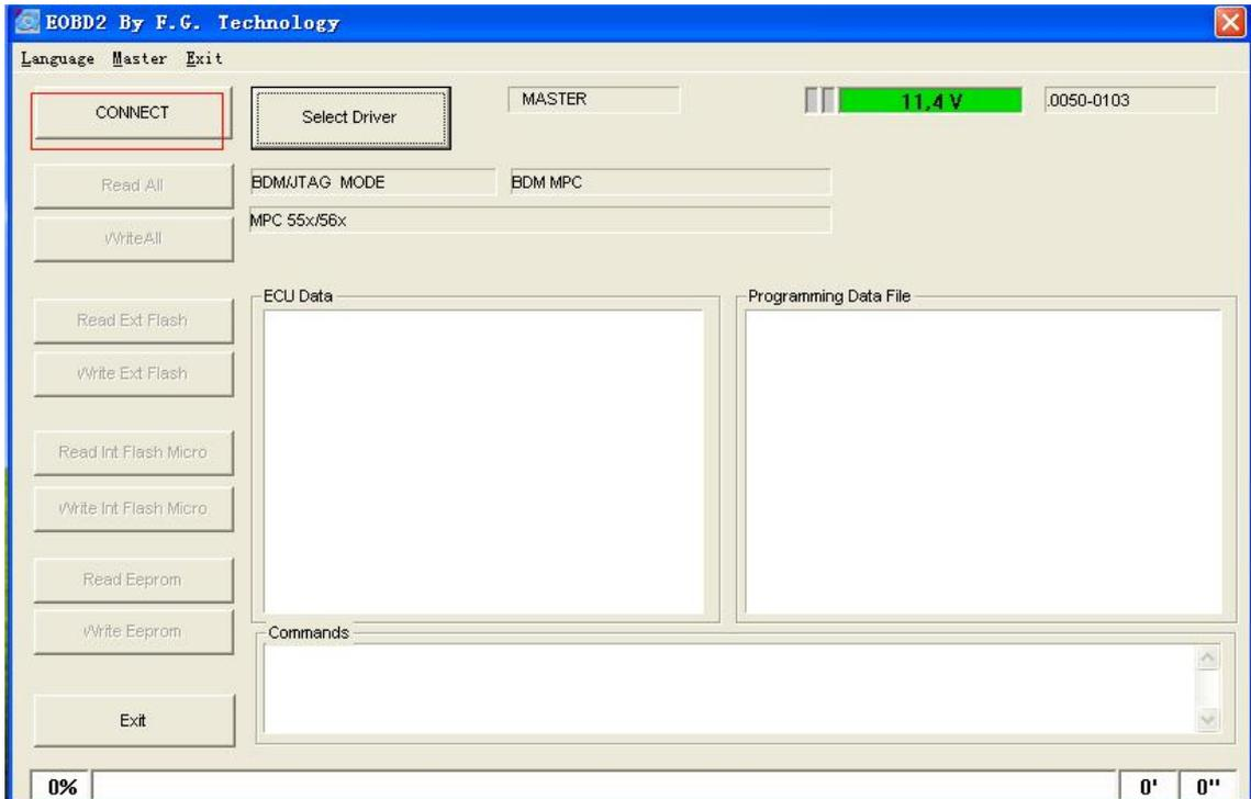
4. After the communication between ECU and the fgtech software, select " Read All " " Read ext flash " " Read Eeprom "
