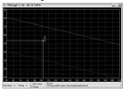
This plug-in allows you to check the injection timing setting on a TDI engine. This needs to be done after you changed the timing belt and every once in a while. The standard procedure for this is to have the engine idling at operating temperature (coolant temp >85\*C), go to measuring block 000 for the engine, switch to basic settings and report fields #2 (injection timing) and #9 (fuel temperature) on a special graph.
