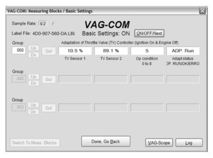
On Controllers using KWP-2000, there is an **[ON/OFF]** button that allows you to initiate and exit Basic Settings while still being able to see the values in the measuring groups.
