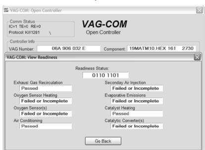
The above screen-shot was taken immediately after clearing the DTC's in a 2000 New Beetle 1.8T. You can see that this car does not support "monitors" for the EGR, Catalyst Heating, or Air Conditioning because this specific car does not have EGR or Catalyst Heating. It does have Air Conditioning, but a "monitor" is only required if the system uses ozone-depleting refrigerant (R12).
