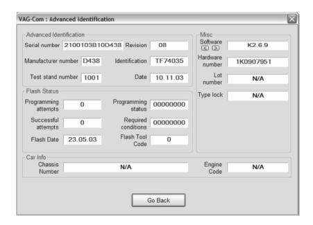
The Advanced ID function is only for control modules using the KWP-2000 Protocol.
