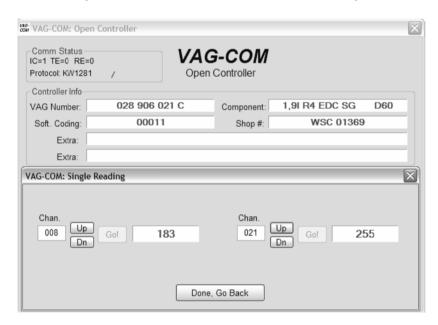
This function allows you to look at real-time data from control modules that support it. However, the data stream coming from the control module gives NO CLUE what the data means or how to scale it into real-world values.
