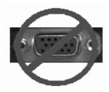
Observe the port we surrounded with the **GREEN** oval. Notice the 9 **MALE** pins? That is a SERIAL port and WILL work! Observe the port circled and crossed in **RED**. Notice the 15 **FEMALE** pins? That is a **MONITOR** port and will NOT work!
