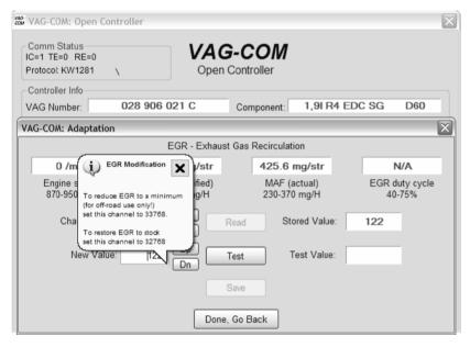
■ Label Files can support values and description for Adaptation channels. A help chart for Adaptation Values may be included in Label Files. If a help chart has been created for an adaptation channel, is displayed in a balloon when you access an Adaptation Channel:
