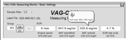
■ Label Files also allow a third label field to be defined for each of the normal measuring block fields. This label is displayed in a balloon when the user clicks on the field. The idea is to put "specified values" in this field:
