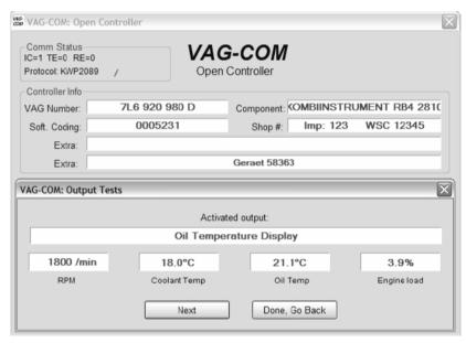
refer to the Factory Repair Manual for your car. Once the Test Sequence has been started, clicking [Done, Go Back] will take you back to the Open Controller Function Screen. THE TEST SEQUENCE WILL STILL BE ACTIVE!
