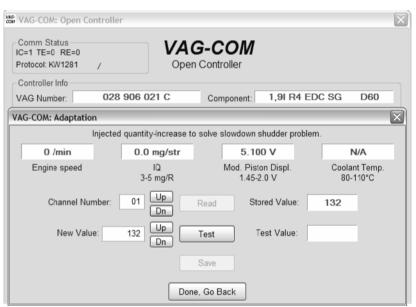
You can use the **[Up]** and **[Dn]** buttons next to *Channel Number* to scroll through all 99 possible channels, or you can manually enter a channel number and click **[Read]**. If a channel exists, VAG-COM will show you the *Stored Value*. If a channel does not exist, the Stored Value will show as "N/A". Other data the controller may or may not send will be decoded and shown in the four display fields at the top of the screen.
