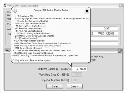
■ Up to 20 lines of coding chart data can be included in a Label File. This data is shown in a balloon on the coding screen.
