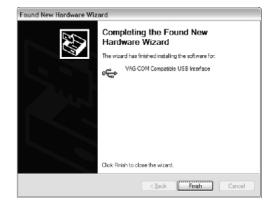
Note: If, for some reason, you installed your USB Interface without following the above instructions, and VAG-COM does not work correctly, go into your PC's Device Manager while the USB Interface is connected. Find the "VAG-COM Compatible USB Interface" and delete it. Then, unplug the USB Interface from your PC, wait 5 seconds and plug it back in. Proceed with the installation starting on Page 2.
