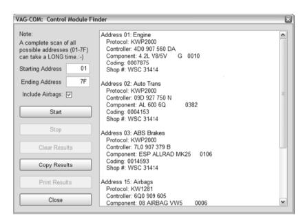
This function cycles through each possible address in the vehicle, finding each controller and reporting its Address, Name, Protocol, Controller VAG Number, Component Number, Soft. Coding, and Work Shop Code.
