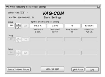
This screen is presented when a Control Module is in Basic Settings Mode.
