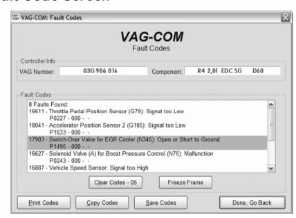
**[Print Codes]** will print a Fault Code Report. If your PC is not connected to a printer when this button is pressed, be sure to use Windows to set the printer to "Work Off-Line" first! Later, when you connect the PC to a printer, un-check "Work Off-Line" to print the report.
