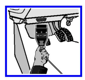
◀ If your vehicle has a 2x2 port (some pre-1996 vehicles), then use a 2x2 Adapter between the Interface and the ports in the car.
