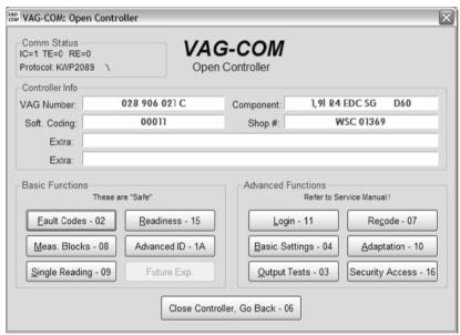
This screen will appear when VAG-COM is attempting to establish communications with any of the Control Modules shown on the Select Control Modules Screen.
