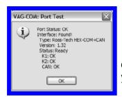
■ Select the correct port for your PC's Serial Port (typically COM1 or COM2) or USB Port (USB) and click the [Test] button. Ensure that VAG-COM finds your interface. You should see a message like this.
