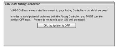
thing that can cause the 65535 DTC to set, we cannot be certain that we have identified everything that could cause it. So the standard warning message will remain in VAG-COM, at least for the time being. In addition, if VAG-COM has any difficulties connecting to the airbag, you may see a screen like this. If you see this screen, please do **exactly** what it tells you!
