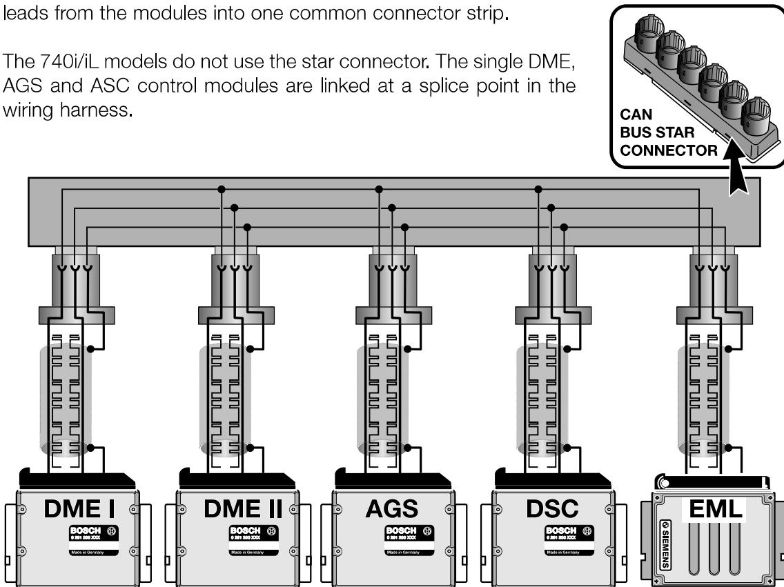
The 1998 model year brought forth the next generation of CAN Bus communicators. The Instrument Cluster and Steering angle sensor of the DSC III system were also linked to the CAN bus to expand the available signalling capabilities.
