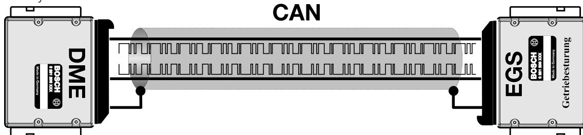
With the introduction of the 1995 750iL, the CAN bus was expanded to include both engine control modules, transmission control module, EML III control module and the DSC II control module.
