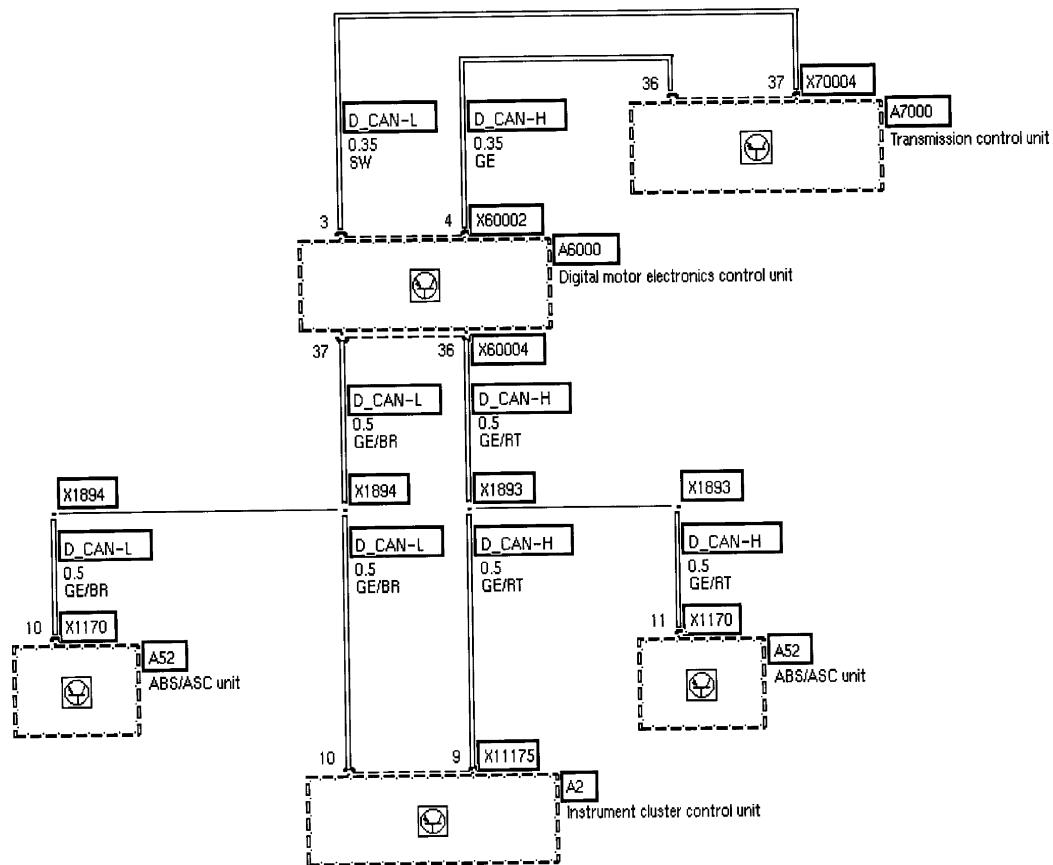
The CAN bus of the 1998 740i/iL and 540i has also changed. The entire CAN bus is twisted pair wiring. The EGS is linked to the DME by a dedicated twisted pair CAN bus with a common twisted pair to all other control modules.
