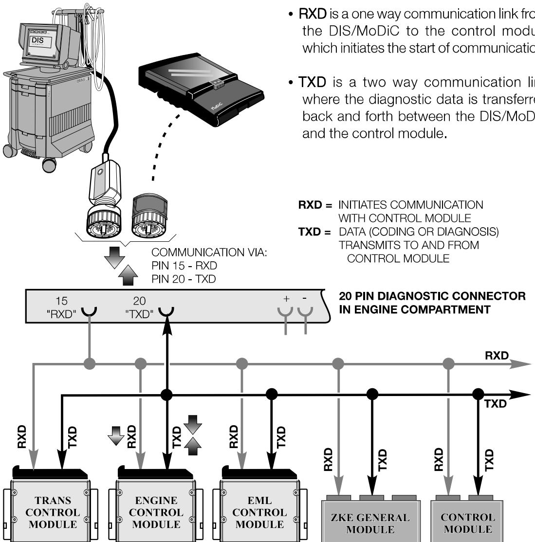
**TXD II:** With the introduction of OBD II, the diagnostic link changed to meet the needs of the OBD II Data Link Connector (DLC). The DLC is located in the passenger compartment and provides a connection for an aftermarket scantool for powertrain systems only. Scantool communication with these control modules is only possible when the 20 pin diagnostic connector cap is installed. A circuit bridge in the cap completes the DLC circuit.
