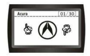
If the vehicle Diagnostic Protocol is OBD-II, But the DTC Code is MANUFACTORY, Please press UP or DN button, then press yes, the screen will change to:
